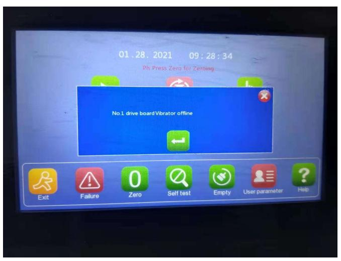
G: Locate the No. 1 drive board, swap VIB1 wire with VIB2 wire.
