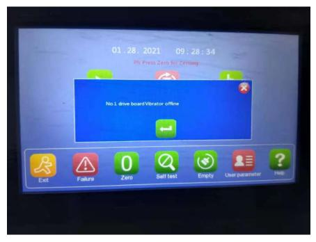
R: Locate No. 1 drive board, confirm if MVP wire is installed properly.
