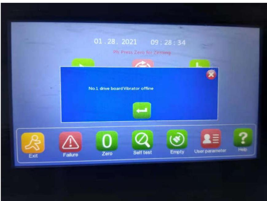
R: Locate No. 1 drive board, confirm if MVP wire is installed properly.
