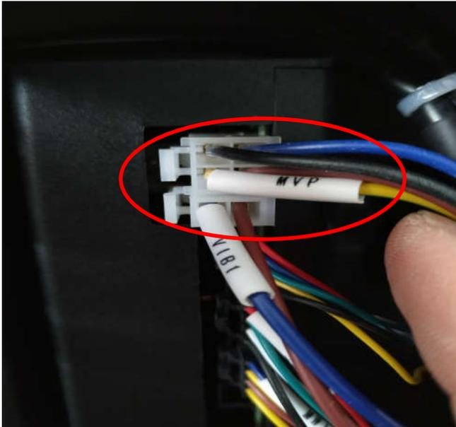
S: Remove MVP wire, confirm if the voltage between brown & yellow wire is AC110V.
