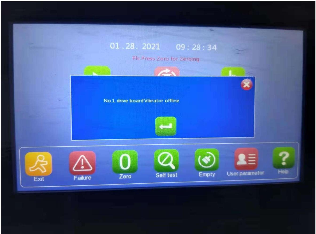
G: Locate the No. 1 drive board, swap VIB1 wire with VIB2 wire.
